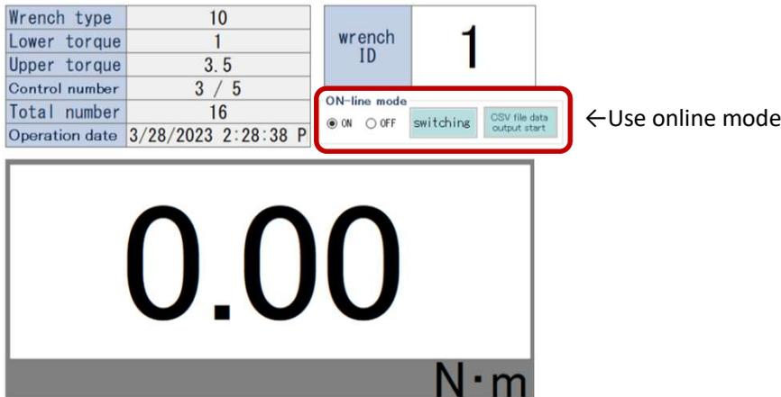
Select "ON" and switch to ON-line mode with the "Switching" button.
