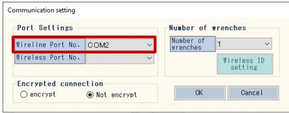
For wireless connections, set the "Wireless Port No.".
