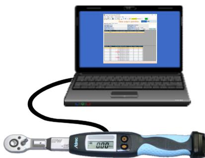
**MEMO mode = Enable** and record the tightening value in the torque wrench body.
