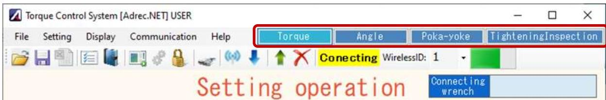
By toggling this button, the item to be set will change. By setting the required items and writing them into the torque wrench, the type of torque wrench can be changed.
