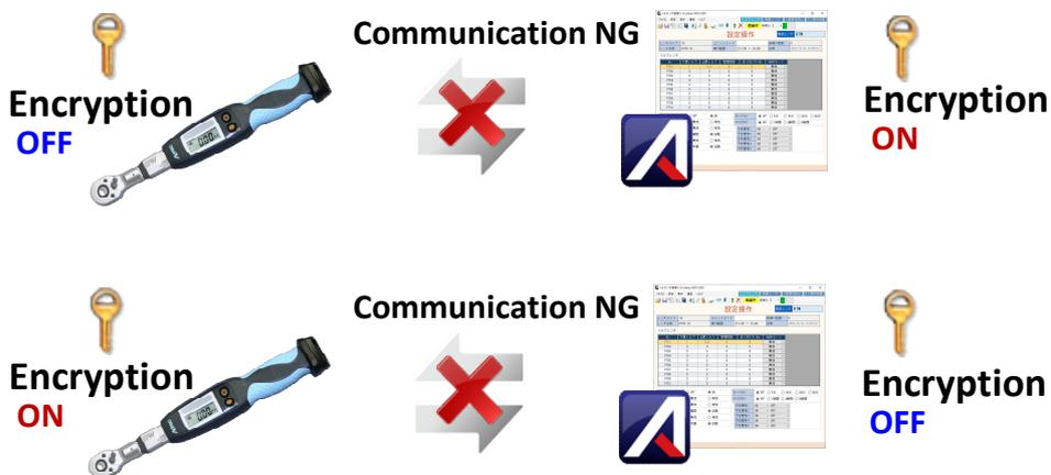
When encrypting, encrypt in the order of Torque Wrench, [Adrec. Net].
