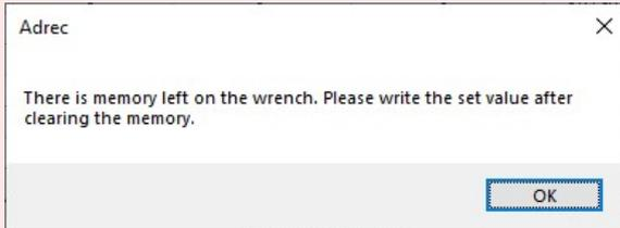
Writing settings to the torque wrench should be done after deleting the record in it from the [Erase Memory Data] icon.
